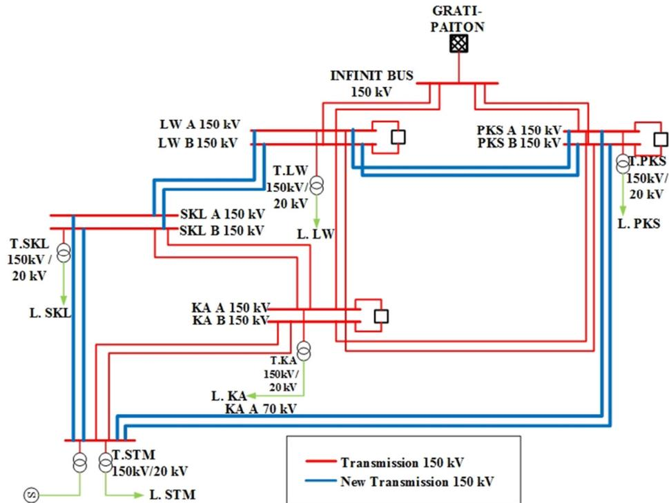
Figure 2. Single Line 150 kV Transmission Line Diagram
