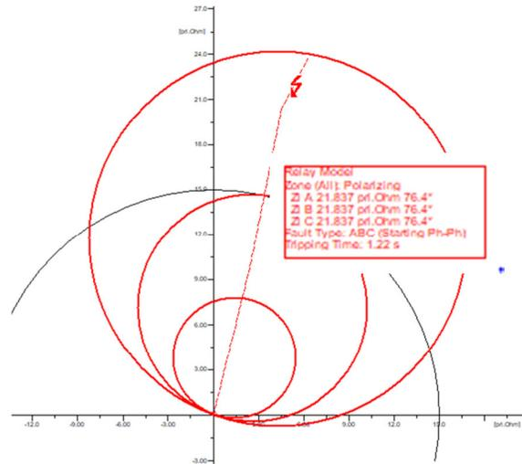
Figure 6. Conditions when disturbances occur in Zone 3 (Sengkaling Substation - Lawang Substation)
