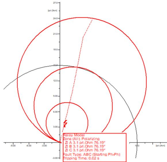
Figure 4. Conditions when disturbances occur in Zone 1 (Substation of Pakis-Substation Sutami)
