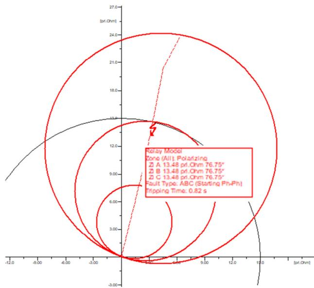
Figure 5. Condition when disturbance occurs in Zone 2 (Sutami substation and Sengkaling substation)
