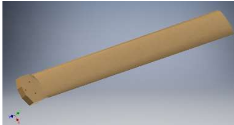
Fig. 15. 3D model of the blade using NACA 4712 airfoil
