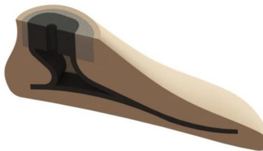
Fig. 4. Assembly of ankle-foot design
