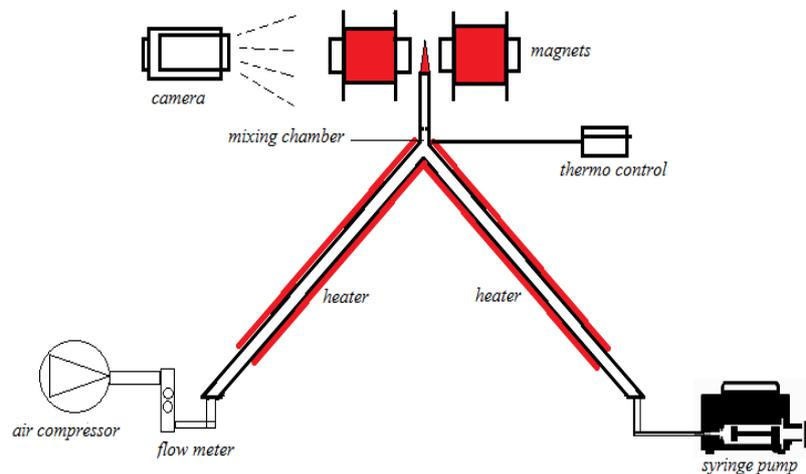
Fig. 1. Bunsen burner research tool schematic
