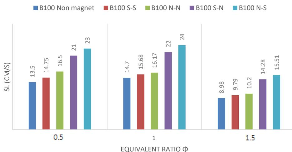
Fig. 5. Laminar burning velocity (SL) fuel B100
