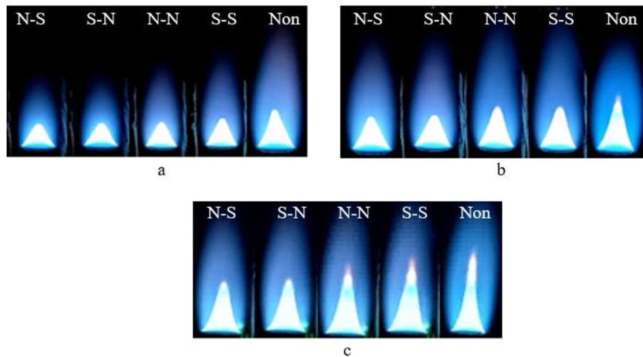
Fig. 3. B100 flame evolution, (a) ratio equivalent 0.5, (b) ratio equivalent 1, (c) ratio equivalent 1.5
