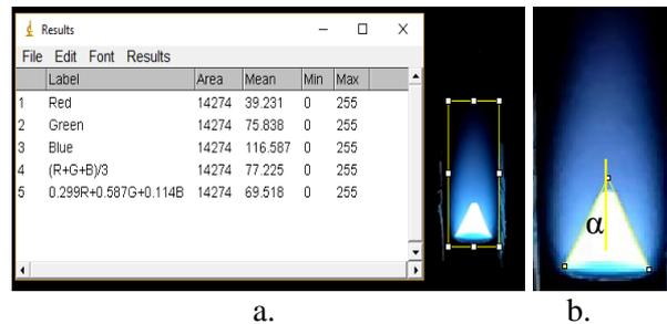
Fig. 2. Data analysis (a). Intensity of RGB color, (b). Flame angle
