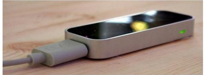
Fig. 2. Leap motion controller
