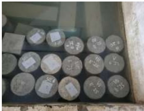
Gambar 11. perawatan beton/curing beton
