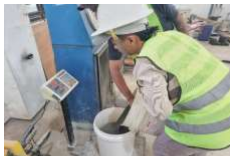
Gambar 7. menimbang material campuran beton
