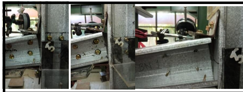
Figure 4.12. Failure in the Screw-Tush-Plate Joint-Angle cleats
