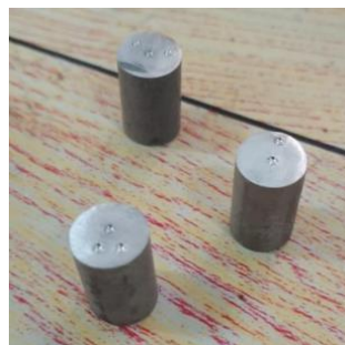
Fig. 4. Hardness testing specimens
