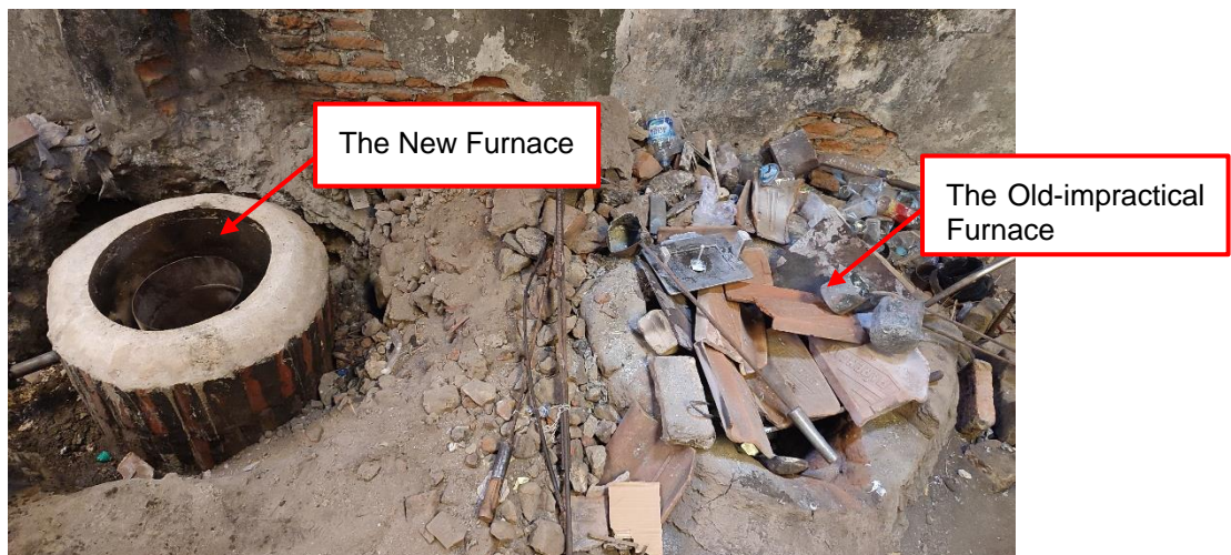
Fig. 11. Image of the new and the old furnace side-by-side
