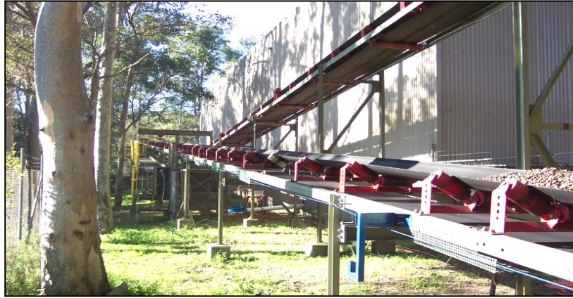
Fig. 1. Idler rolls are shown in operation on a typical belt conveyor [9].
