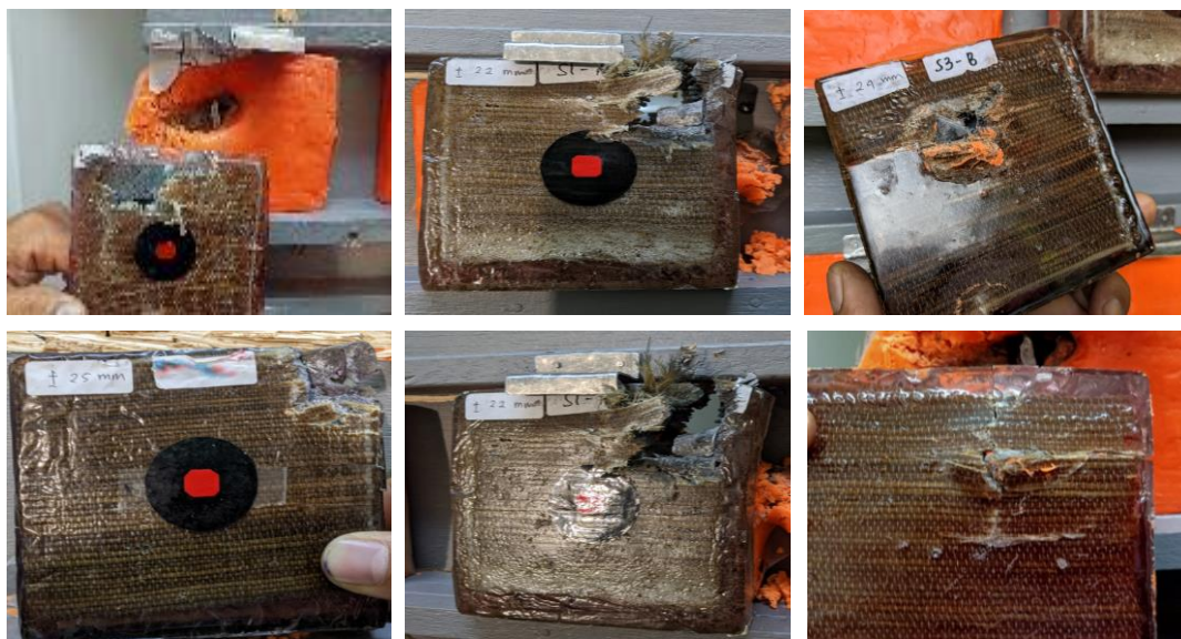
Fig. 7. Multilayer panel specimens not able to withstand bullet penetration
