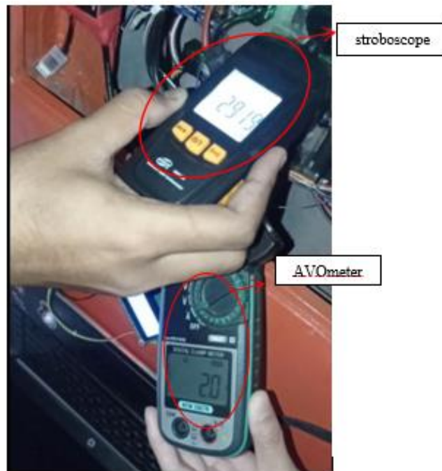
Fig. 8. DC brushless motor testing
