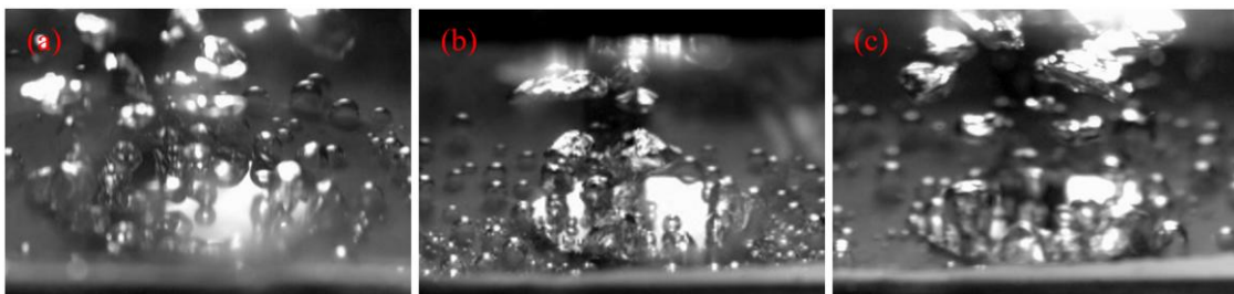
Fig. 13. Surface visualization: (a) test specimen C at \dot{q} = 37.03 \text{ kW/m}^2 , (b) test specimen C-1 at \dot{q} = 37.1 \text{ kW/m}^2 , and (c) test specimen C-2 at \dot{q} = 42.68 \text{ kW/m}^2
