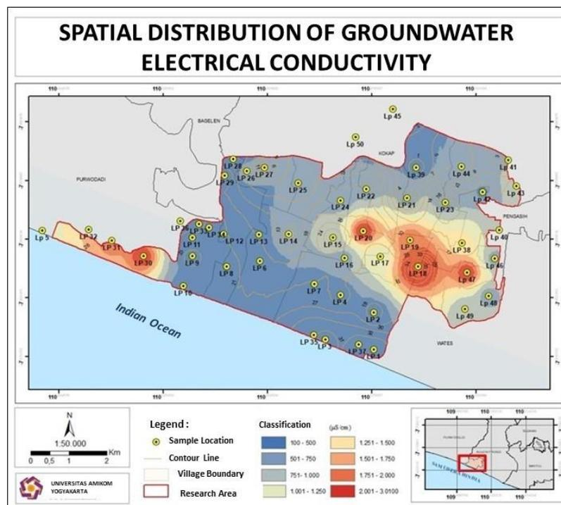
Figure 3. Distribution of Groundwater Electrical Conductivity
