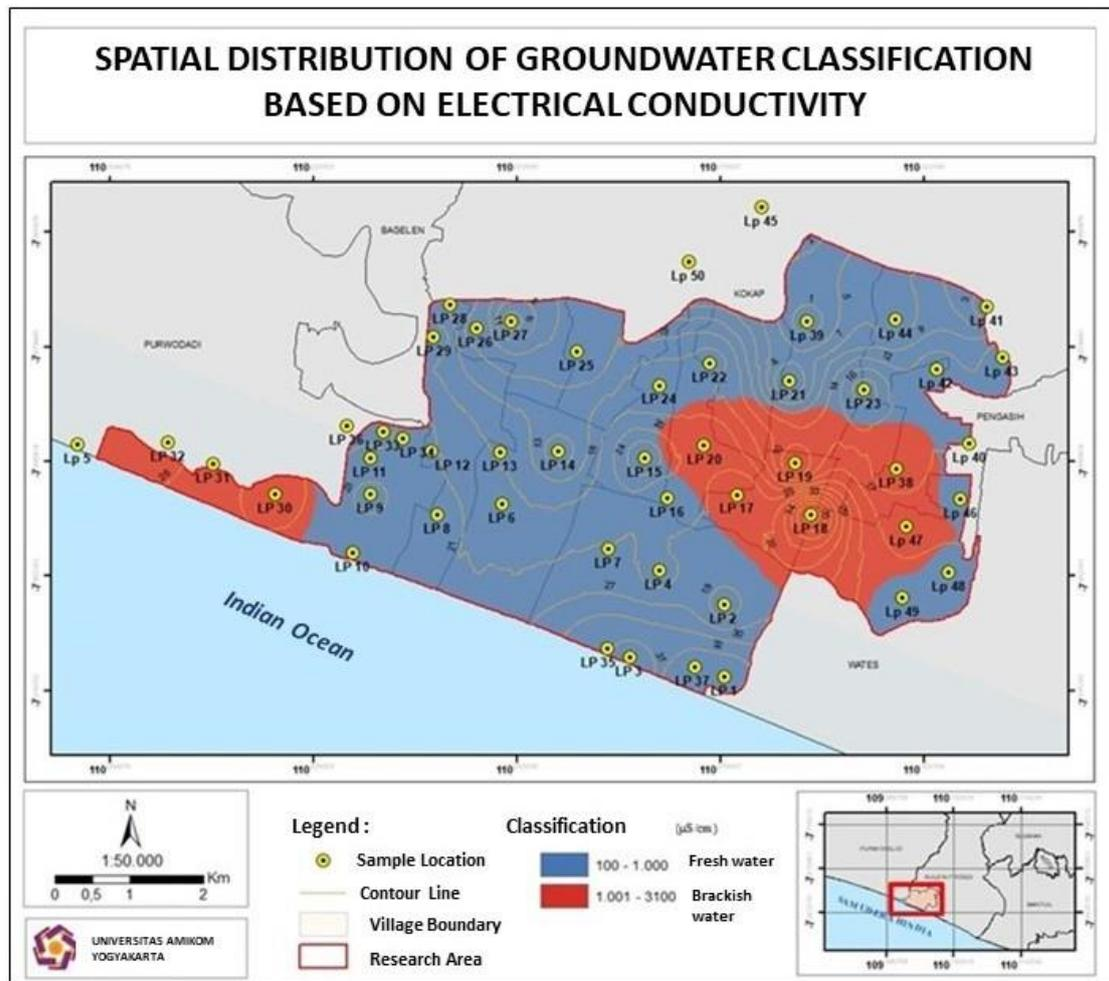
**Figure 5. Groundwater Distribution based on Electrical Conductivity**
