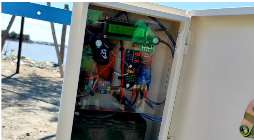
Figure 17. Charge controller integration test.
