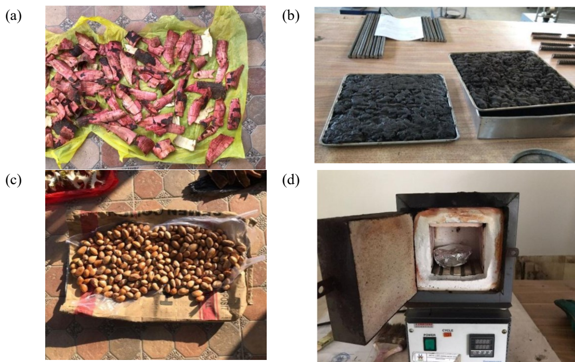
Figure 1. (a) cassava peel (b) spent bleaching earth (c) durian seed (d) carbonization process
