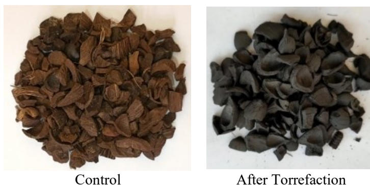
Figure 2. Palm Kernel Shell Before and After Torrefaction Process
