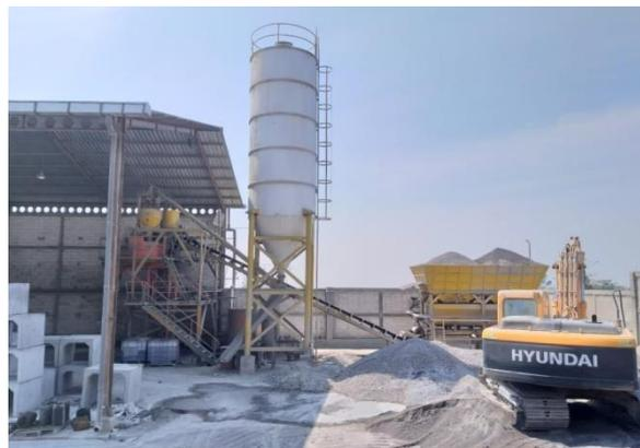
Gambar 1. Mesin *Batching Plant*
