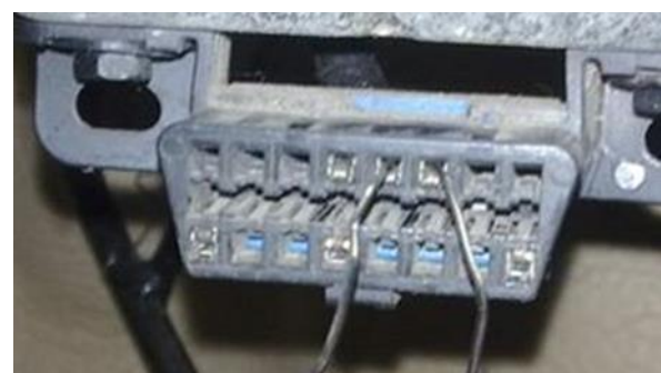
Gambar 12. Pengecekan CAN Bus
