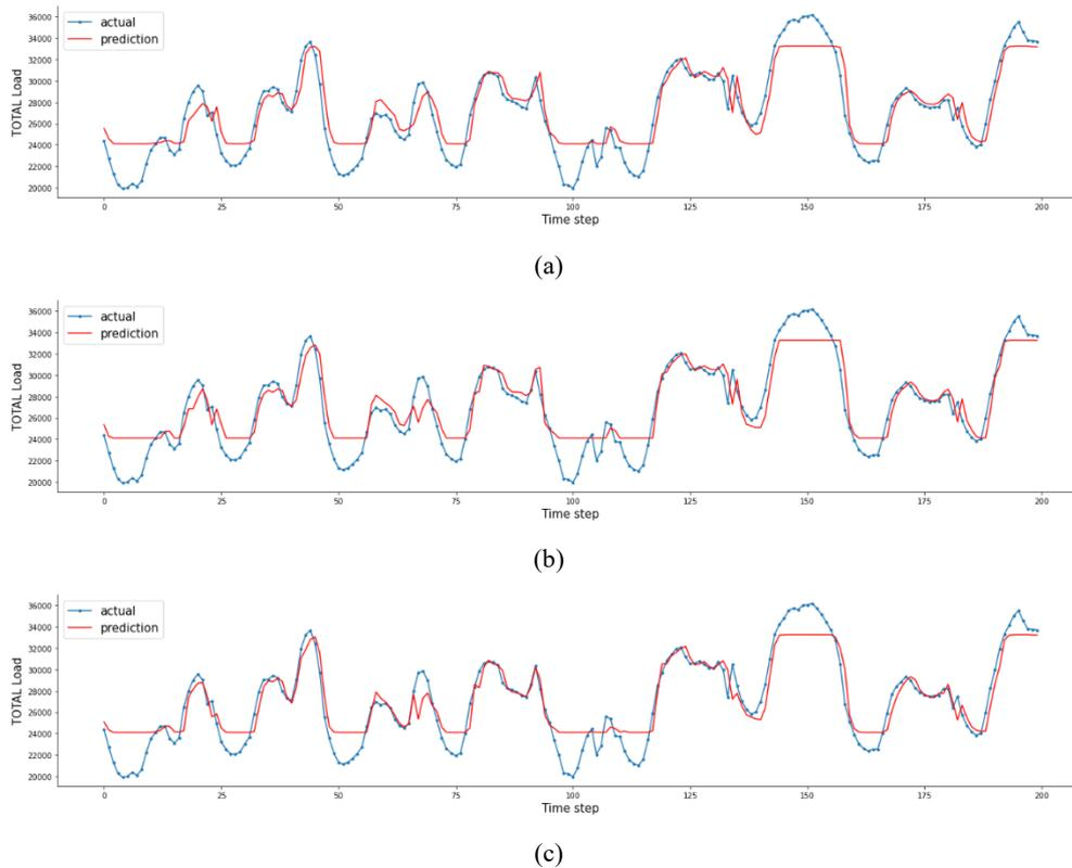
Fig. 4. Attention LSTM's configuration (Z-Score normalization): (a) Att-LSTM, (b) Att-Grid Search-LSTM, and (c) Att-PSO-LSTM
