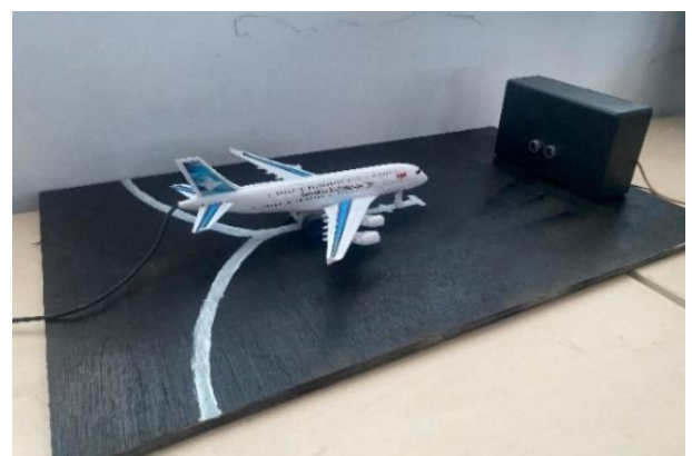
Fig. 3. Actual Setup of The Sensor and NodeMCU ESP32 On A Mock-Up Aircraft
