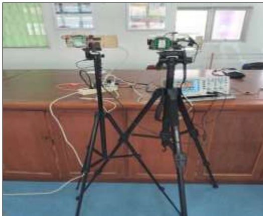
Gambar 4. Array prototipe radar Doppler X-band
